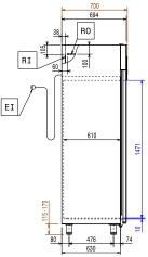
Electrical inlet (power) Refrigerant Inlet RI R0 = Refrigerant Outlet
